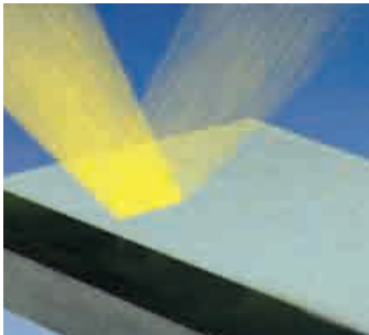
Cleaning process stops when target material is removed
