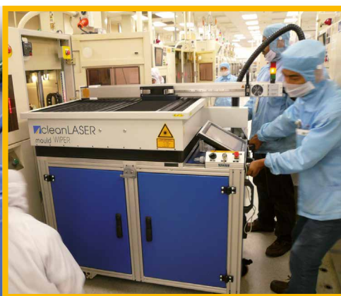
Fully automated mobile „moldWIPER“ cleaning system
