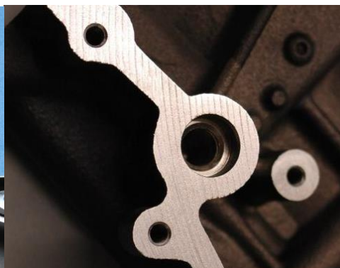
Sealing contour with preserved milling structure after laser processing
