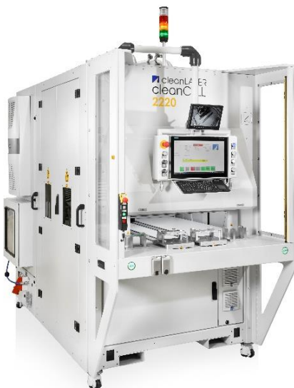
Customized cleanCELL 2220 for seal pre-treatment of aluminum control housings
