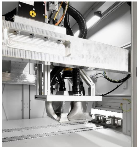
Sealing pre-treatment of an aluminum housing with a 4-suction nozzle concept for optimum removal of the emerging particles
